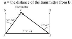
The measure of angle *CBA* is  $90^{\circ} - 53^{\circ}40' = 89^{\circ}60' - 53^{\circ}40' = 36^{\circ}20'$ . The measure of angle *CAB* is  $90^{\circ} - 36^{\circ}20' = 89^{\circ}60' - 36^{\circ}20' = 53^{\circ}40'$ .  $A + B = 90^{\circ}$ , so  $C = 90^{\circ}$ . Thus, we have  $\sin A = \frac{a}{2.50} \Rightarrow \sin 53^{\circ}40' = \frac{a}{2.50} \Rightarrow a = 2.50 \sin 53^{\circ}40' \approx 2.0140$
