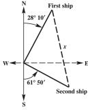
The angle between the bearings of the ships is  $180^{\circ} - (28^{\circ}10' + 61^{\circ}50') = 90^{\circ}$ . The triangle formed is a right triangle. The distance traveled at 24.0 mph is (4 hr) (24.0 mph) = 96 mi. The distance traveled at 28.0 mph is (4 hr) (28.0 mph) = 112 mi. Applying the Pythagorean theorem we have  $x^2 = 96^2 + 112^2 \Rightarrow x^2 = 9216 + 12,544 \Rightarrow x^2 = 21,760 \Rightarrow x = \sqrt{21,760} \approx 147.5127$
