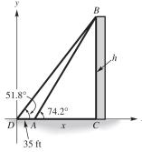
Superimpose coordinate axes on the figure with D at the origin. Thus, the coordinates of A are (35, 0). The tangent of the angle between the x-axis and the graph of a line with equation y = mx + b is the slope of the line. For line DB,  $m = \tan 51.8^{\circ}$ . Because b = 0, the equation of line DB is  $y_1 = x \tan 51.8^{\circ}$ . The equation of line AB is  $y_2 = x \tan 74.2^{\circ} + b$ . Use the coordinates of A and the point-slope form to find the equation of AB.
