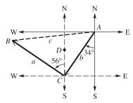
The port is at A. Because the NS lines are parallel, the measure of angle  $ACD = 34^{\circ}$ . Therefore, the measure of angle  $ACB = 34^{\circ} + 56^{\circ} = 90^{\circ}$ , making triangle ABC a right triangle. The ship traveled at 18 knots for 2.5 hours or 18(2.5) = 45 nautical miles from A to C, labeled b in the figure. The ship traveled at 18 knots for 3.0 hours or 18(3.0) = 54 nautical miles from C to B, labeled C in the figure. Use the Pythagorean theorem to find the distance from C to C
