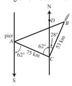
Angle *ACB* is a right angle, so use the Pythagorean theorem to find the distance from *A* to *B*.
