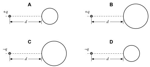
Rank the force exerted on the point charge by the sphere (let a force to the right be a positive force and a force to the left be a negative force).
