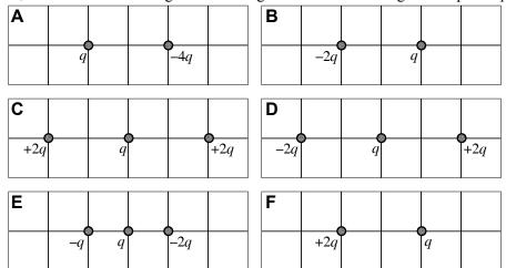
Rank the magnitude of the electric force on the charge labeled q due to the other charges.
