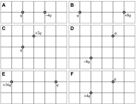
Rank the magnitude of the electric force on the charge labeled q due to the other charge.
