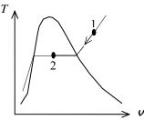
**3-60** The water in a rigid tank is cooled until the vapor starts condensing. The initial pressure in the tank is to be determined.
