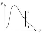
**3-34E** Left chamber of a partitioned system contains water at a specified state while the right chamber is evacuated. The partition is now ruptured and heat is transferred to the water. The pressure and the total internal energy at the final state are to be determined.
