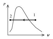
3-39 A piston-cylinder device that is filled with R-134a is heated. The final volume is to be determined.
