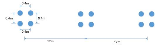
a. Determine the inductance per phase in mH/km (40 points).
