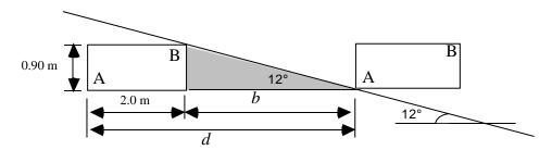
The distance d is equal to the length of the window plus the base of the 12° right triangle of height 0.90 m.
