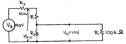
For a loading error of 0.1%, the voltage drop across  $R_s$  should be  $90 \times 0.001 = 0.09$  V. The current through  $R_s$  is then:
