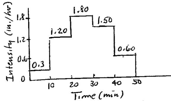
To convert the depths to intensities, divide by the interval and include conversion factors; for example,  $(0.05 \text{ in./10 min.}) * (60 \text{ min./hr.}) = 0.30 \text{ in./hr.}$
