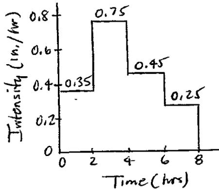
To convert the depths to intensities, divide the depths by the time interval; for example,  $0.7 \text{ in./2 hr.} = 0.35 \text{ in./hr.}$
