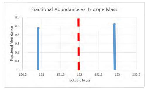
In a mass spectrometer experiment, the two blue solid lines would appear in the mass spectrum of an elemental europium sample. In contrast, it is the x-value of the dotted red line which is presented in the periodic table of atomic weights for europium.
