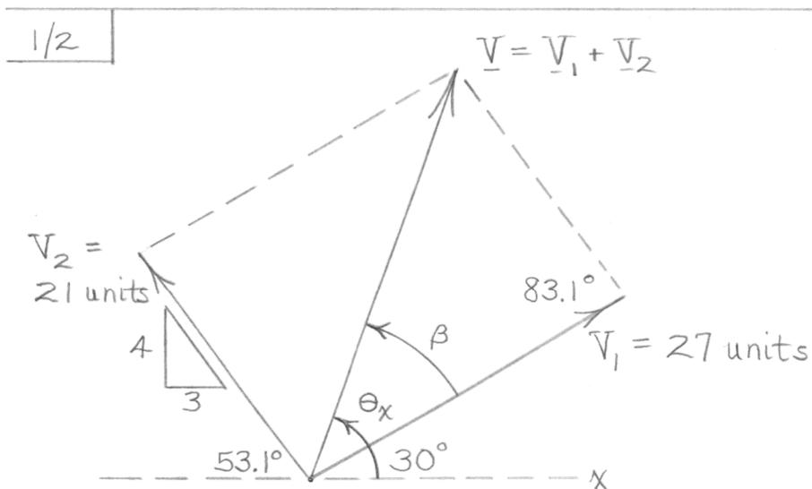
Graphically,  $\underline{V} = \underline{32 \text{ units}}$ ,  $\theta_x = \underline{70^\circ}$
