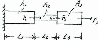
$$P_1 = 4 \text{ kN} \quad L_1 = 0.6 \text{ m} \quad A_1 = 2 \times 10^{-4} \text{ m}^2$$
