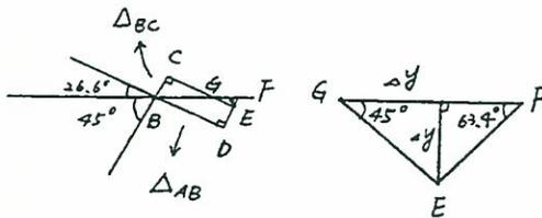
$$\begin{aligned} \Delta y &= \sqrt{2} \times \Delta_{AB} - \Delta x \\ &= \sqrt{2} \times 0.007321 - 0.00375 \\ &= 0.009978 \text{ in} \end{aligned}$$
