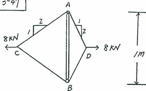
$$T_{AD} = T_{DB} = 8.94 \text{ kN}$$
