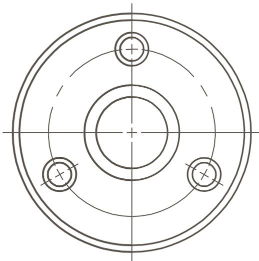
Ⓓ Using a trammel, sketch the missing symmetrical half of the object.
