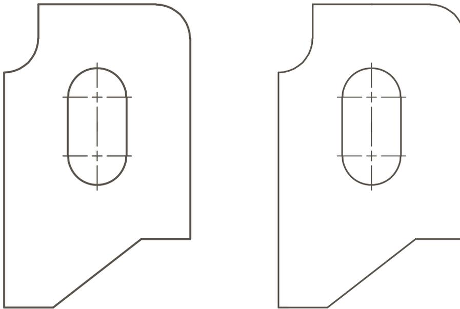
(A) Using a trammel, sketch the missing symmetrical half of the object.
