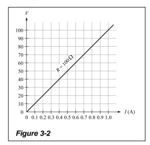
The graph is a straight line as shown in Figure 3-2. This indicates a *linear* relationship between *I* and *V*.
