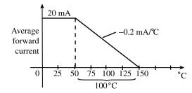
$$\frac{0.2 \text{ mA}}{^{\circ}\text{C}} = \frac{20 \text{ mA}}{x}$$
