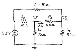
$$\frac{v_1 - 25}{R_2} + \frac{v_1}{R_4} + \frac{v_1 - v_2}{R_3} = 0$$
