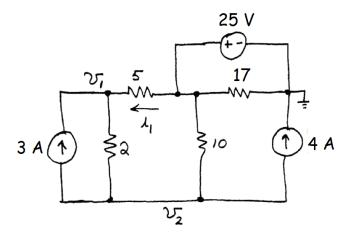
$$\frac{v_1 - 25}{5} + \frac{v_1 - v_2}{2} = 3$$
