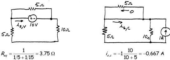
$$i_{s,v} = -\frac{10 \text{ V}}{R_{eq}} = -2.667 \text{ A}$$
