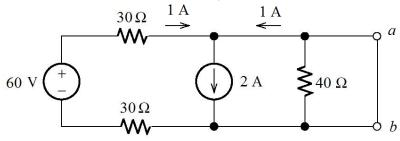
Thus, the short-circuit current is 1 A flowing out of b and into a. Zeroing the sources, we have
