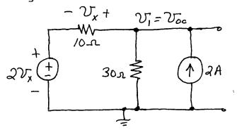
$$\frac{v_{\text{oc}} - 2v_{x}}{10} + \frac{v_{\text{oc}}}{30} = 2 \qquad v_{\text{oc}} = 3v_{x}$$
