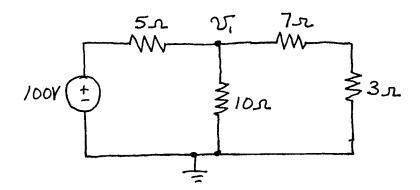
The node equation is  $(v_1 - 10)/5 + v_1/10 + v_1/10 = 0$ . Solving we find that  $v_1 = 50$  V. Thus we again find that the current through the  $10-\Omega$  resistance is  $i = v_1/10 = 5$  A.
