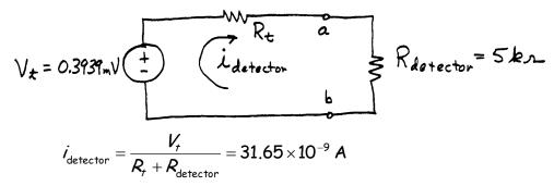
Thus, the detector must be sensitive to very small currents if the bridge is to be accurately balanced.
