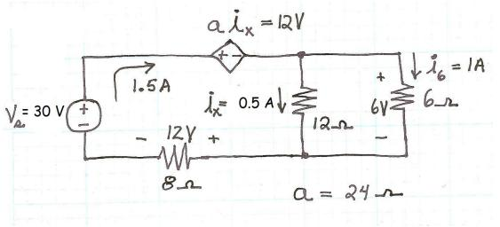
However, the circuit actually has  $V_s = 10$  V, so the actual value of  $i_6$  is  $\frac{10}{30} \times (1 \text{ A}) = 0.3333 \text{ A}.$
