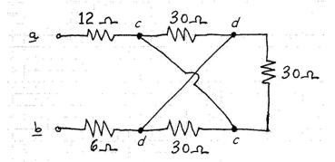
Notice that the points labeled c are the same node and that the points labeled d are another node. Thus, all three of the 30- $\Omega$  resistors are in parallel because they are each connected between nodes c and d. The equivalent resistance is 28  $\Omega$ .
