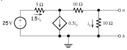
Using KVL, we have  $25 = 5(1.5i_x) + 10i_x + 10i_x$  Solving, we find  $i_x = 0.90909$  A and then we have  $V_t = v_{oc} = 10i_x = 9.0909$  V.
