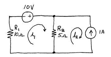
current  $\it i_2$  as the current referenced downward through the current source. However, we know that the current through this source is 1 A flowing upward. Next we write a
