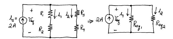
$$R_{eq1} = R_1 + R_2 = 20 \Omega$$
