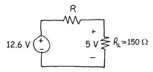
Applying the voltage-division principle, we have  $12.6 \frac{150}{150 + R} = 5$ . Solving, we find  $R = 228 \Omega$ .
