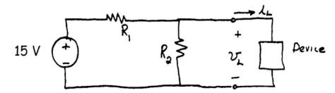
With  $i_L=0$  and  $v_L=5\,V$ , we must have  $\frac{R_2}{R_1+R_2}\times 15=5\,V$ . Rearranging, this gives
