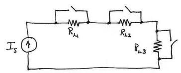
To turn a load on, we open the corresponding switch, and to turn a load off, we close the switch.
