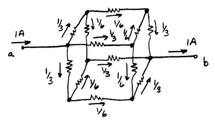
Then, the voltage between terminals a and b is
