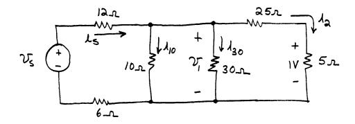
$$i_2 = (v_2/5) = 0.2 \text{ A}$$
