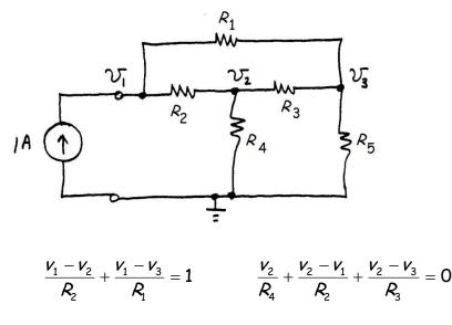
$$\frac{v_3}{R_5} + \frac{v_3 - v_1}{R_1} + \frac{v_3 - v_2}{R_3} = 0$$
