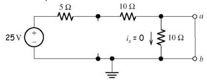
$i_{sc}=\frac{25}{15}=1.667$  A. Then, we have  $R_t=v_{oc}/i_{sc}=5.45\,\Omega$ . Thus, the equivalents are:
