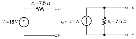
Then, maximum power is obtained for a load resistance equal to the Thévenin resistance.
