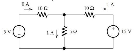
We see that the 5-V source produces 25% of the total current through the 5- $\Omega$  resistance. However, the power produced by the 5-V source with both sources active is zero. Thus, the 5-V source produces 0% of the power delivered to the 5- $\Omega$  resistance. Strange, but true! Because power is a nonlinear function of current (i.e.,  $P = Ri^2$ ), the superposition principle does not apply to power.
