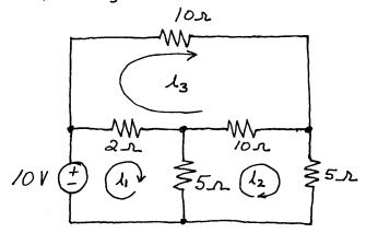
Then we write KVL equations following each mesh current:
