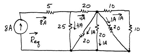
P2.26\* We combine resistances in series and parallel until the circuit becomes an equivalent resistance across the voltage source. Then, we solve the simplified circuit and transfer information back along the chain of equivalents until we have found the desired results.
