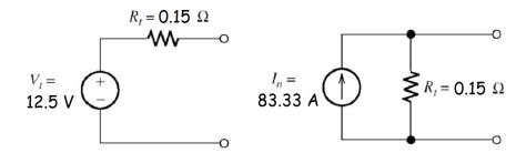
The short-circuit current is 83.33 A. Because no energy is converted from chemical form to heat in a battery under open-circuit conditions, the Thévenin equivalent seems more realistic from an energy conversion standpoint.
