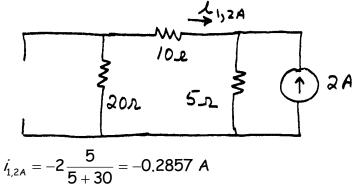
Finally,  $\dot{i_1} = \dot{i_{1.1A}} + \dot{i_{1.2A}} = 0.2857 A$
