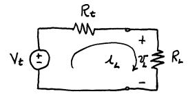
For a load of 1 k $\Omega$ , we have  $i_L = 8/1000 = 8$  mA , and we can write  $v_L = V_t - R_t i_L$ . Substituting values this becomes  $8 = V_t - 0.008 R_t$  (1)
