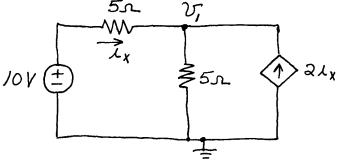
Then use  $i_x = (10 - v_1)/5$  to substitute and solve. We find  $v_1 = 7.5$  V.
