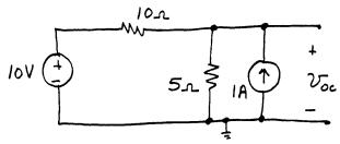
$$\frac{v_{oc} - 10}{10} + \frac{v_{oc}}{5} = 1$$
