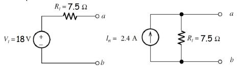
Notice the source polarity relative to terminals a and b.
