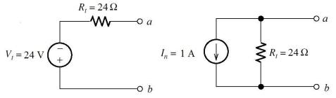
Because the short-circuit current flows out of terminal b, we have oriented the voltage polarity positive toward b and pointed the current source reference toward b.
