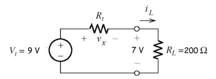
We have  $i_L = \frac{7}{200} = 35 \, \text{mA}$  and  $v_x = V_t - 7 = 2 \, \text{V}$ . Thus, the Thévenin resistance is  $R_t = \frac{2 \, \text{V}}{35 \, \text{mA}} = 57.14 \, \Omega$ .
