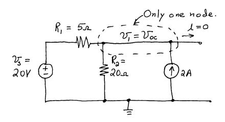
Notice that the node voltage is the open-circuit voltage. Then write a KCL equation:
