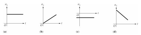
The acceleration can be described as follows: (a) positive and constant, (b) positive and increasing, (c) negative and constant, (d) positive and decreasing.
