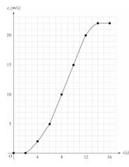
**Reflect:** The acceleration is constant when the velocity changes at a constant rate. When the velocity is constant, the acceleration is zero.
