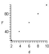
24. Hooke's Law states that the force F required to compress or stretch a spring (within its elastic limits) is proportional to the distance d that the spring is compressed or stretched from its original length. That is, F = kd where k is the measure of the stiffness of the spring and is called the *spring constant*. The table below shows the elongation d in centimeters of a spring when a force of F kilograms is applied.
