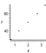
24. Hooke's Law states that the force F required to compress or stretch a spring (within its elastic limits) is proportional to the distance d that the spring is compressed or stretched from its original length. That is, F = kd where k is the measure of the stiffness of the spring and is called the *spring constant*. The table below shows the elongation d in centimeters of a spring when a force of F kilograms is applied.
